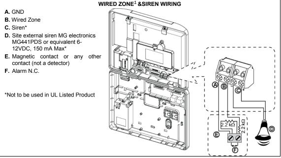
Figure 4.4 – Wired Zone and Siren Wiring
