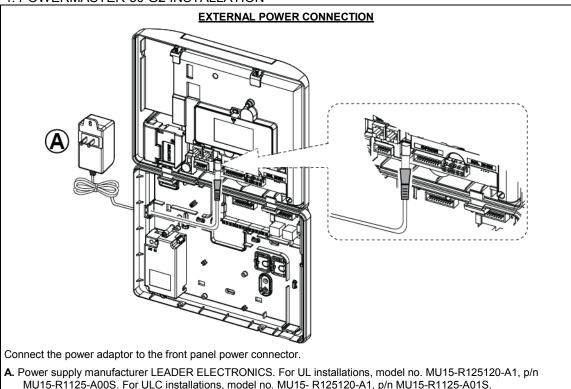
Figure 4.10b – External Power Connection
