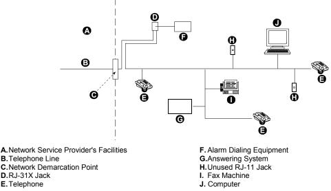
Note: The REN is used to determine the number of devices that may be connected to a telephone line. Excessive RENs on a telephone line may result in the devices not ringing in response to an incoming call. In most but not all areas, the sum of RENs should not exceed five (5.0). To be certain of the number of devices that may be connected to a line, as determined by the total RENs, contact the local telephone company.
