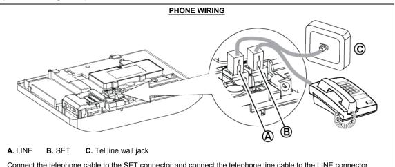
Connect the telephone cable to the SET connector and connect the telephone line cable to the LINE connector (through the desired wiring cable entry).
