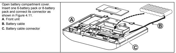
Figure 4.11 – Battery Insertion
