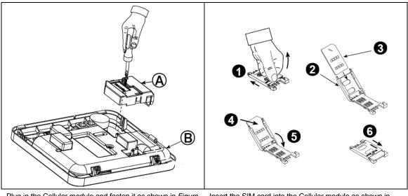
Plug in the Cellular module and fasten it as shown in *Figure* 3.4 above.
