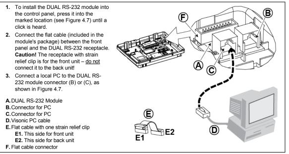
Figure 4.7 – Dual RS-232 Module Mounting
