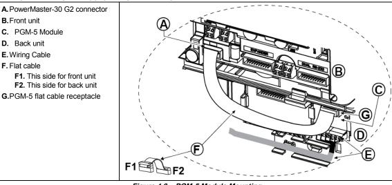
Figure 4.8 – PGM-5 Module Mounting
