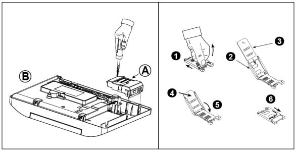
Plug in the GSM module and fasten it as shown in the above drawing.
